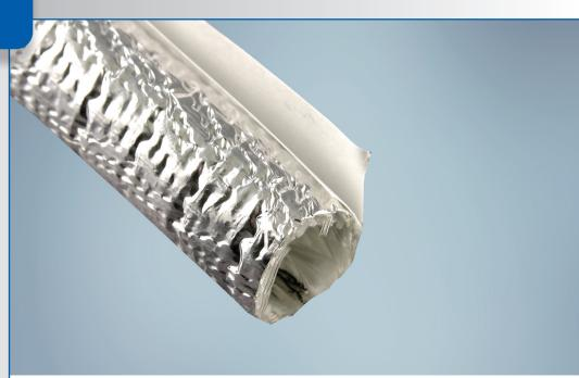
Therm-L-Wrap™66 is a self-wrapping, reflective sleeve designed to provide thermal protection from both radiant and convective heat. Composed of a woven fiberglass base fabric and a lamination of aluminum foil, the product can withstand convective heat soaks up to 200°C and simultaneously protect critical components from radiant or reflected heat.
